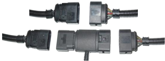
Photo 2. Connection of the adaptor to the VP-37 pump interface.
